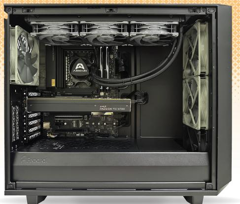
month based on an AMD Ryzen 9 7950X. Its Cinebench R23 multithread rendering result of 38,611 was the fastest in the £4,500 category, and the Blender rendering time of 265 seconds was also top in this class. The OpenCL-accelerated Adobe Media Encoder time of 105 seconds beat every other system this month.
